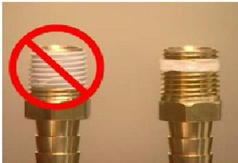
Picture 7 – proper application of sealant
