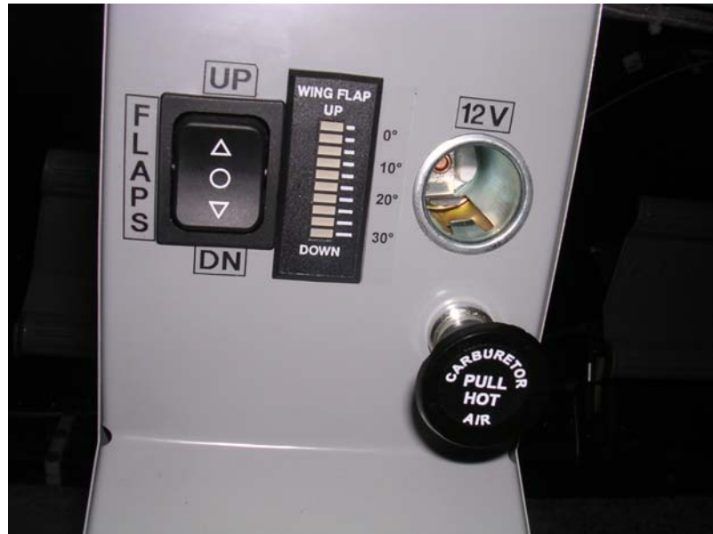
PICTURE 1 – LED Flaps position indicator
